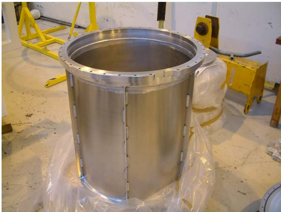
Here is the large vacuum tank (700mm bore), plus adaptor ring.
